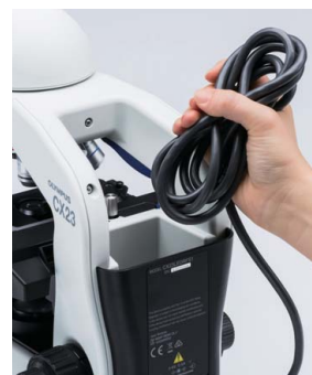
Cable storage compartment
